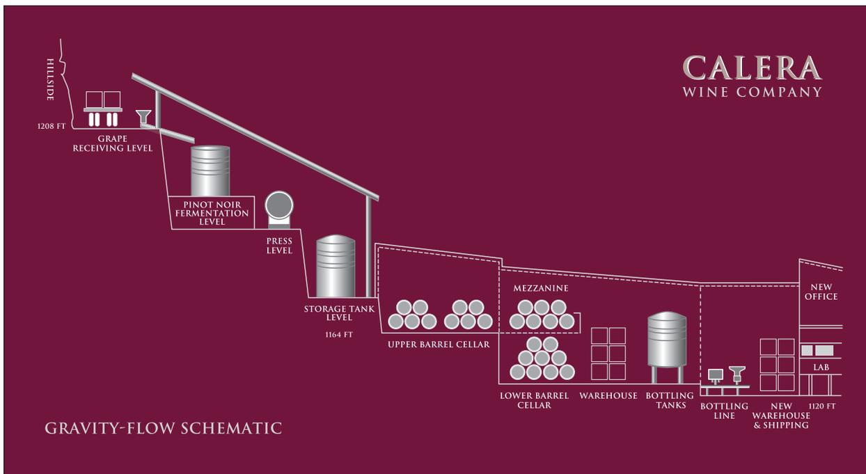
Seven levels allows for extremely gentle handling of the grapes and wine. Pumps which could damage the fruit or harm the wine are rarely used.
